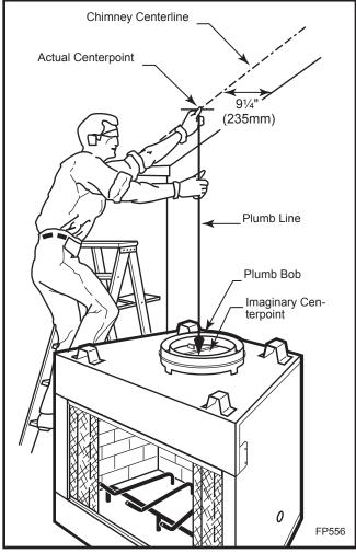
Fig. 11 Locate centerline of chimney with plumb line.
